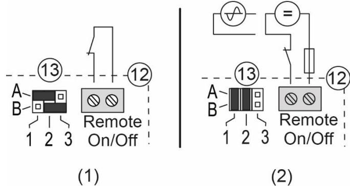
**Control by dry contact:** the jumpers remain in their original position (1) A1-2 and B2-3.
