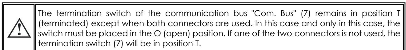
The max accumulated length of the communication bus is 300m. Due to a line voltage drop, it is
