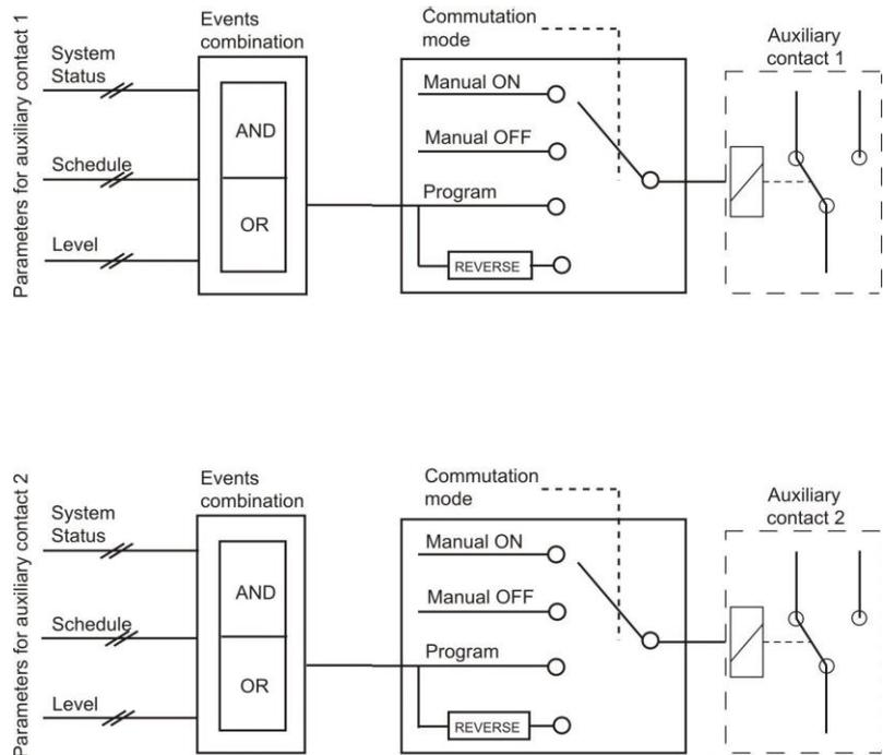
The auxiliary contacts react to different types of signals, graphically illustrated below. Basic events that activate the contacts are:
